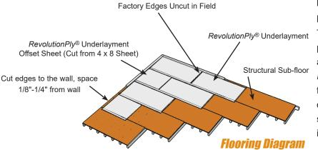
lightly butt the panels together without applying any pressure so they barely touch at the joints.
